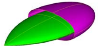
CAD model of the coated NASA almond
